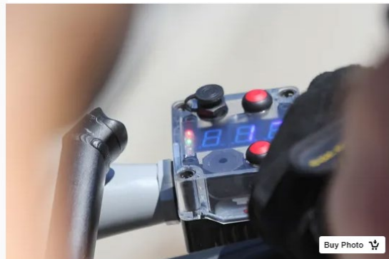
This device, called a C3FT and pronounced as "see three feet," will be used on two Knoxville Police Department bicycles to measure the distance between the bikes and passing cars. (Photo: Ryan Wilusz/News Sentinel)
